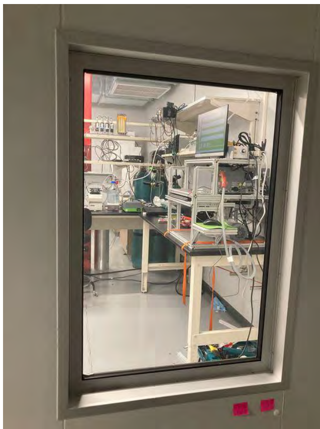
Figure II-9. Picarro laser spectrometer and custom-built vaporizer and standardization system built by UW being installed in OSU COLDEX laboratory (June 7 2023). View from inside the CFA freezer.
