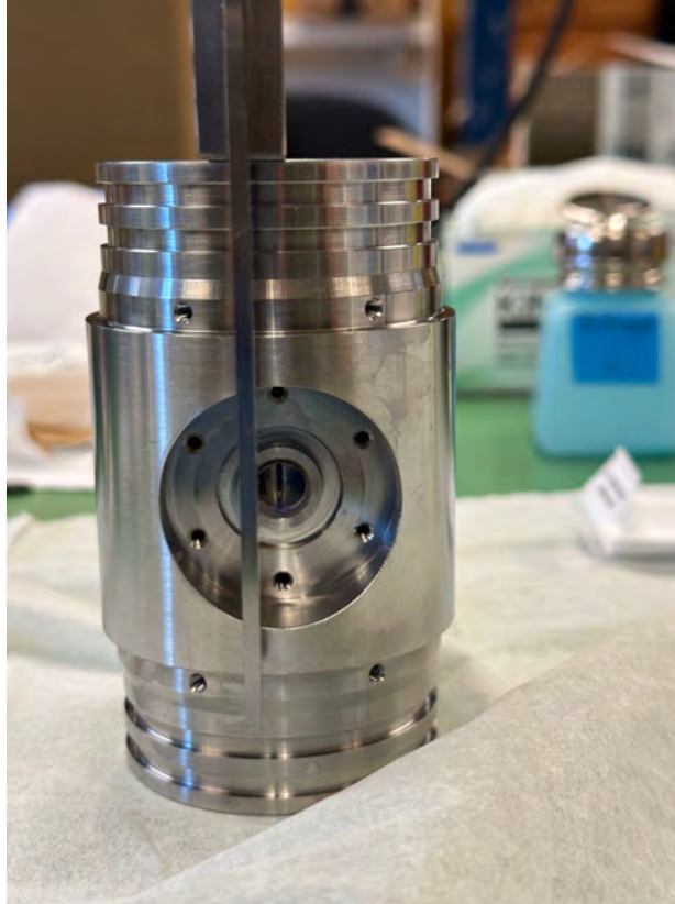
Figure II-6. New Ice Diver section to include a sapphire optical port for the dust-logger laser.
