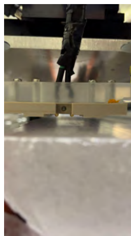
Figure II-12. DC electrodes on ICF ECM system are gold-plated spring-loaded balls that improve ice contact by rolling as the measurements are made along the core.
